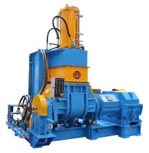
**Overview** Standard Dispersion Kneader is categorized in the closed system mixer. It is being used for mixing different materials together. The advantages of a closed system mixer is that it is able to control the temperature and chemical waste during the mixing process. As a result, the mixing is more efficient and faster.
