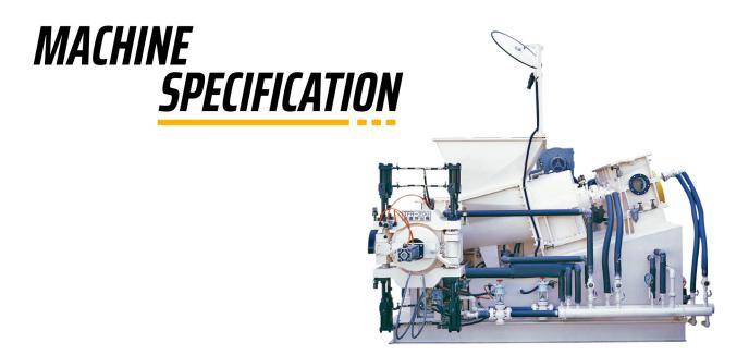
**Overview** It is a machine consisting of a spiral worm which rotates in the barrel. As for the worm and barrel threads, the temperature can be set as needed. The rotation of the worm screw will cause the compound to continuously enter the barrel and create pressure for the compound to flow through the die in the front to form a shape.
