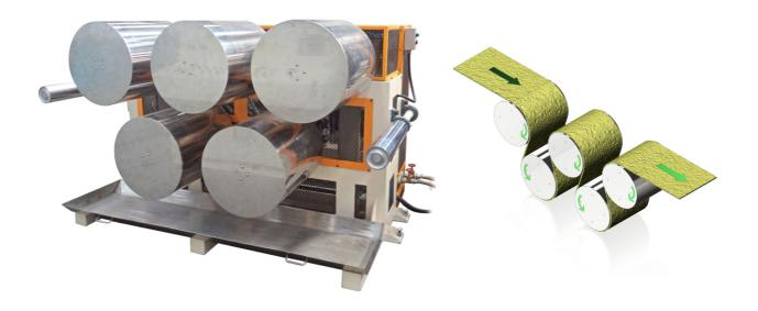
**Overview** As same as the batch off series, this cooling roller machine is a rubber cooling machine which is consisted of 5 - 7 rolls. They are special rolls that have cooling water flowing inside them. Therefore, once the rubber sheet run through this cooling rolls, it will be cool-off and ready for the cutting process.
