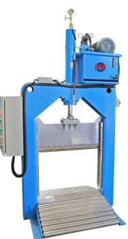
**Overview** There are two types of rubber bale cutter which are RBS and RBN cutter. The functions are quite the same. However, the RBN is more suitable for cutting heavy and large size of rubber bales.
