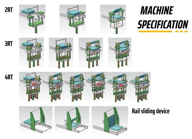
**Overview** Compressor is a product forming machine which uses 2 or more plates of mold, which are pressed by hydraulic system. When the pressure is being transferred to the mold, compound rubber will be forced to fill up the empty space of the mold, and the heat from the mold will cause the rubber to become stable.
