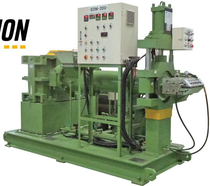
**Overview** It is a machine consisting of a spiral worm which rotates in the barrel. As for the worm and barrel threads, the temperature can be set as needed. The rotation of the worm screw will cause the compound to continuously enter the barrel and create pressure for the compound to flow through the die in the front to form a shape.
