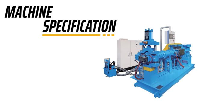
**Overview** It is a machine consisting of a spiral worm which rotates in the barrel. As for the worm and barrel threads, the temperature can be set as needed. The rotation of the worm screw will cause the compound to continuously enter the barrel and create pressure for the compound to flow through the die in the front to form a shape.
