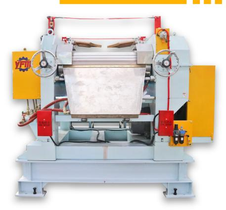
**Overview** The 3-Roller Mixing Mill is an open system mixer consisting of 3 rollers arranged horizontally in parallel. Rolling at different speeds. The mixing process will begins with the rubber being put in between the rollers.
